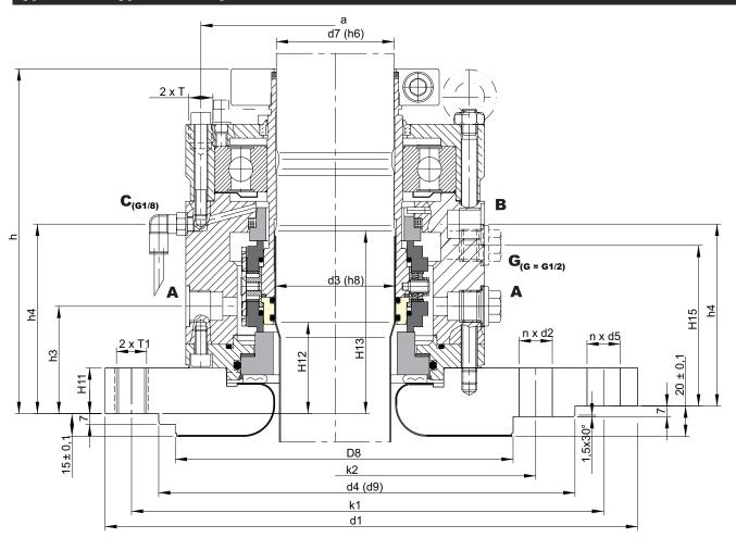
CK736 Liquid lubricated CK736 D Dry running, easy barrier gas supply with dry nitrogen
