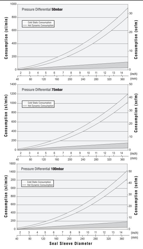
Shaded areas indicate expected consumption ranges for typical application conditions. Actual consumption is dependent on application speed, temperature and individual installation.
