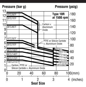
The maximum operating speed for seals up to 75mm/3in shaft diameter is 4,000 rpm: above 75mm/3in. the limit is 1,500 rpm. Type 10R silicon carbide face inserts must not be used at a velocity greater than 7.5m/s/1,500 fpm.
