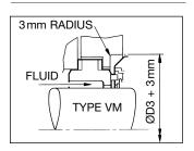
Seat type VM for seal sizes 16 to 25mm/0.750 to 1.000in. is used to promote increased fluid flow to the seal faces.
