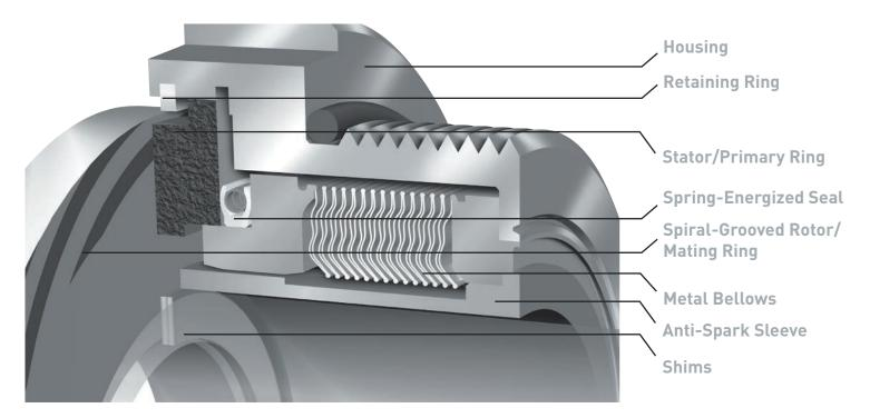
Our commitment to the advancement of the industries we support helps us to ensure peak performance from your equipment even in the toughest applications. Type 285 can safely seal the most common industrial liquid gases, such as liquid nitrogen, oxygen, argon and carbon dioxide and meets liquid oxygen (LOX) safety standards. Combining non-contacting technology with a customized metal bellows design, guarantees safe and dependable performance from the Type 285 across all operating conditions.
