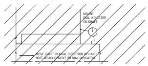
3. Check the squareness or face runout of the seal chamber face to the shaft. The maximum value should not exceed 0.0005" per inch of seal chamber bore diameter. F.I.M.
