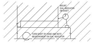
4. Measure the concentricity of the seal chamber bore to the shaft. This value should not exceed 0.005" F.I.M.
