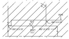
2. Measure the shaft end float/end play. The maximum value should notexceed 0.005" F.I.M.. Remove all sharp edges and burrs over which the seal sleeve must pass.
