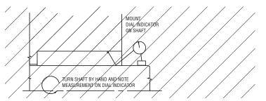
5. Measure the shaft runout at the seal location. The maximum value should not exceed 0.001" F.I.M.
