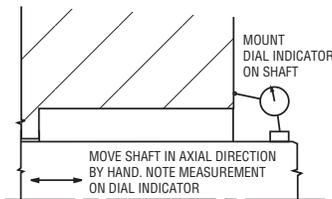
3. Determine squareness of seal chamber face to shaft (0.001mm per mm/.001" per inch of shaft diameter F.I.M. max.), and shaft concentricity to the seal chamber.
