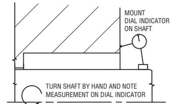
4. Measure shaft runout (0.001mm per mm/.001" per inch of shaft diameter F.I.M. max.).
