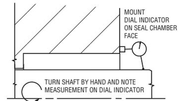
**NOTE:** If measured dimensions exceed those values given, correct the equipment to meet specifications prior to seal installation.
