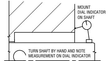
4. Measure shaft runout (0.05mm/0.002" FIM max.).
