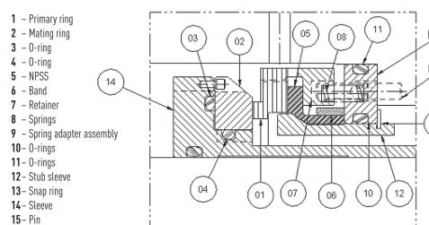
The 8648SC secondary containment seal is sized on known equipment dimensions used in pipeline applications. Sizes to fit common pipeline pumps up to 6.500 inch shafts.
