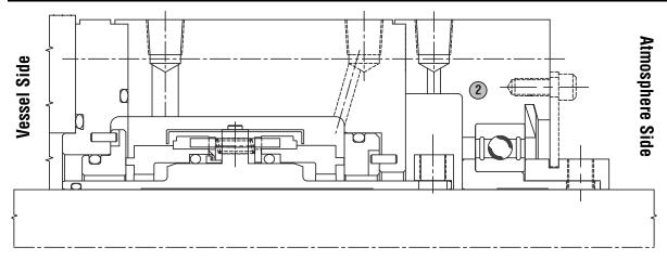
The bearing housing (2) is a modular option available where additional shaft stability is desired.
